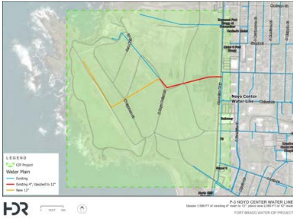
Figure 36 – CIP Project P-3: Noyo Center Water Line
